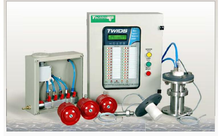
TWIDS consists of a control panel and a set of two water detectors in each hold. An audio / visual alarm is annunciated in case of water ingress in any hold / dry space. The control panel provides individual indication for status, fault & alarm for each cargo hold with distinct signals for pre & main alarm levels.
