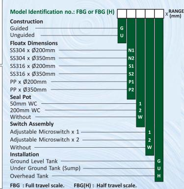
FBG can be installed on tank "when empty" or "in service" Additional Information to be provided: Range x Service liquid x Temp. x Pressure
